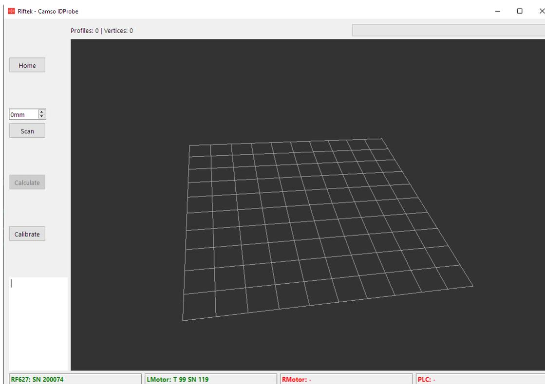
Set the scanning height in mm. Start the measurement process by clicking the **Scan** button.
